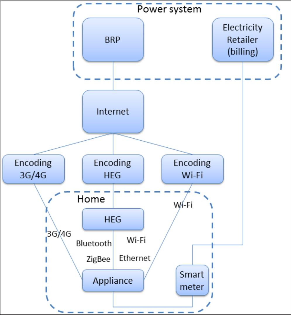
Figure 4: Principle of communication transfers between supply and demand side
