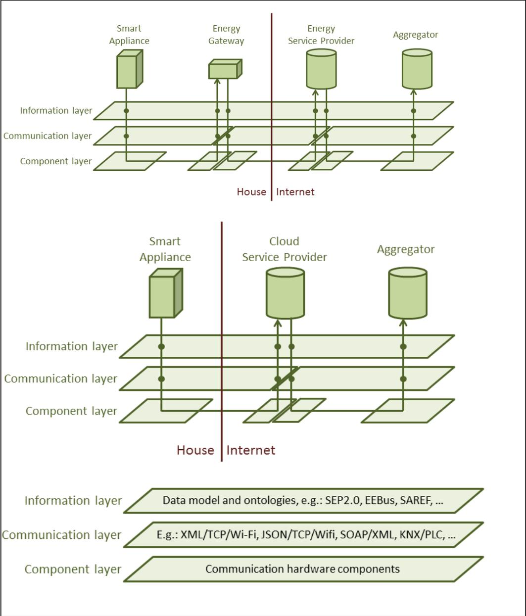
Figure 5: Details of communication transfers, with BRP split up in service provider and aggregator
